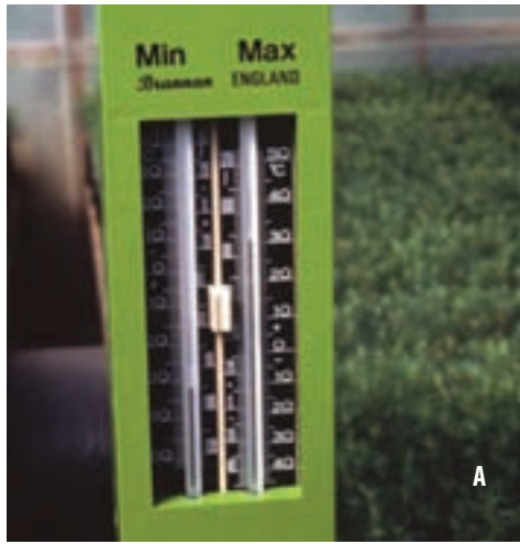
Figure 4.17 —(A) Monitoring and controlling temperature is critical to successfully growing a crop of native plants, and monitoring equipment is inexpensive. Many nurseries use thermometers that record daily maximum and minimum temperatures and (B and C) small, programmable, self-contained temperature sensors. Photo A by Thomas D. Landis, B and C by David Steinfeld.
