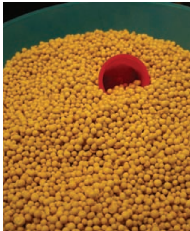
Figure 11.7 —Polymer-coated fertilizers occur as round “prills” in which nutrients are encapsulated by a plastic coating that controls the rate of nutrient release. Photo by Douglass F. Jacobs.
