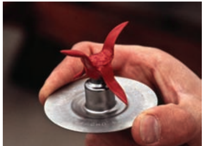
Figure 7.15 —Modifying kitchen blender blades by using rubber coating allows the grower to clean small lots of dry and fleshy fruits without damaging the seeds. Photo by R. Kasten Dumroese.
