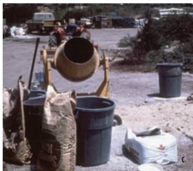
Figure 5.10 —(A) Nurseries that mix their own media should first screen materials and then (B) mix them thoroughly using the moving pile technique. (C) To reduce labor, a cement mixer can also be used but care must be taken to avoid overmixing and the resultant damage to particle size and structure. Photos A and B by Thomas D. Landis, C by Tara Luna.
